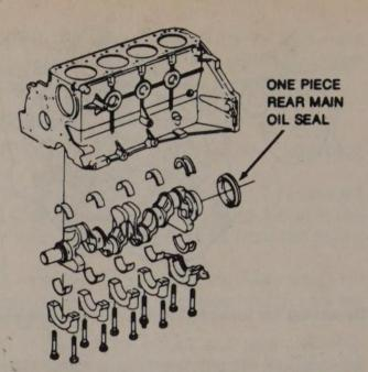
The four cylinder has a one piece ring type rear main seal
