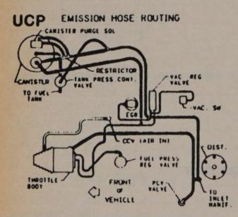
1985 6–2.8L engine (VIN S) without AIR pump
