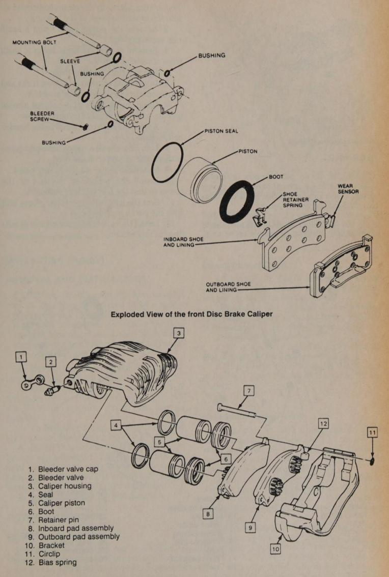
Double piston front caliper
