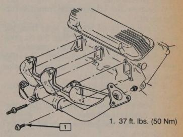
Right exhaust manifold - 3.8L Turbo
