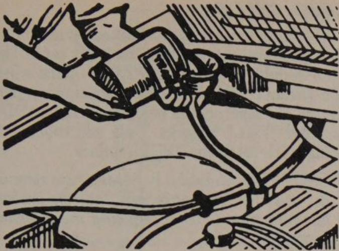
Add automatic transmission fluid through the dipstick tube
