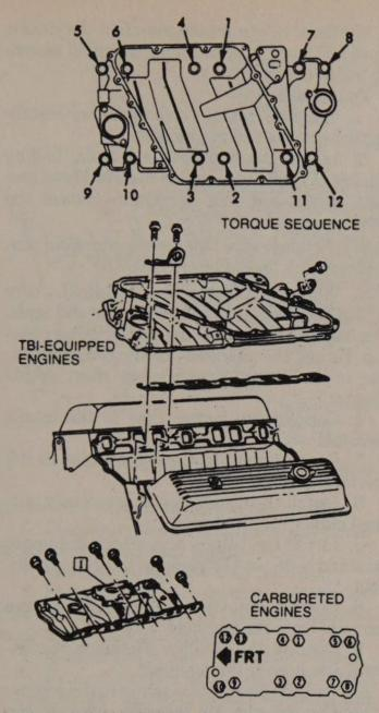
Intake manifold bolt tightening sequence of all Chevrolet-built V8 engines. Note that the lower sequence is used for all carbureted engines, whereas the upper sequence is used for all TBI-equipped engines
