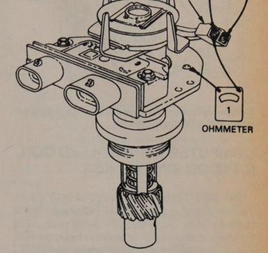
Pickup coil testing – Test 1, should read infinite at all times. Test 2, should read .500–1500 ohms
