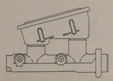
The fluid should be level with the top of the observation windows
