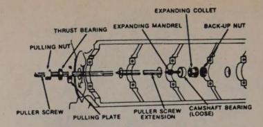
Camshaft bearing removal and installation tool
