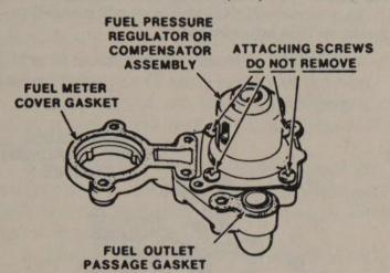
Bottom view of the fuel meter cover assembly – do not remove the four screws indicated
