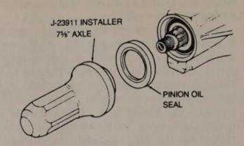
Rear axle pinion oil seal installation
