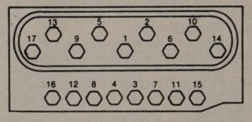
Tightening sequence for the 5.0L engine cylinder head
