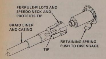
Speedometer cable-to-instrument cluster removal
