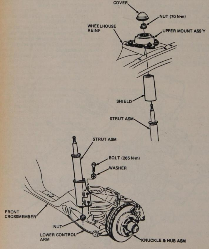
**Remove or install strut**
