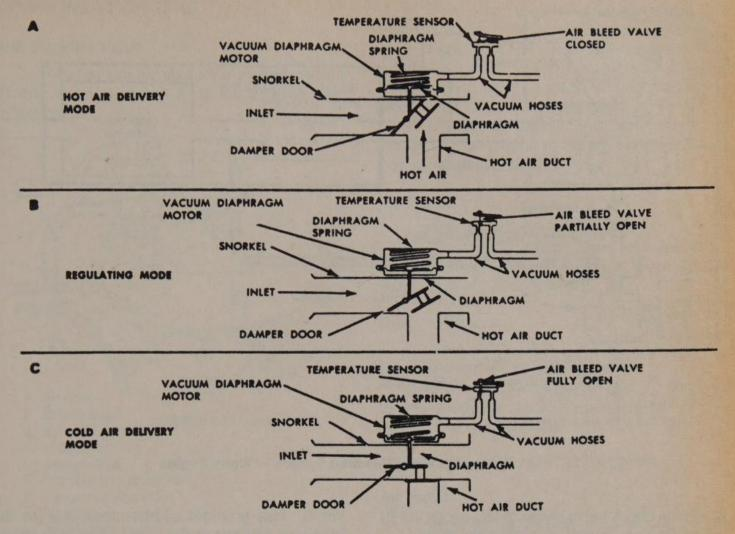
Schematic of the vacuum motor operation
