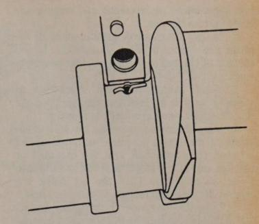
Removing upper crankshaft bearing
