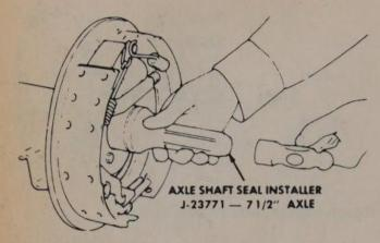
Installing the Rear Axle Seal
