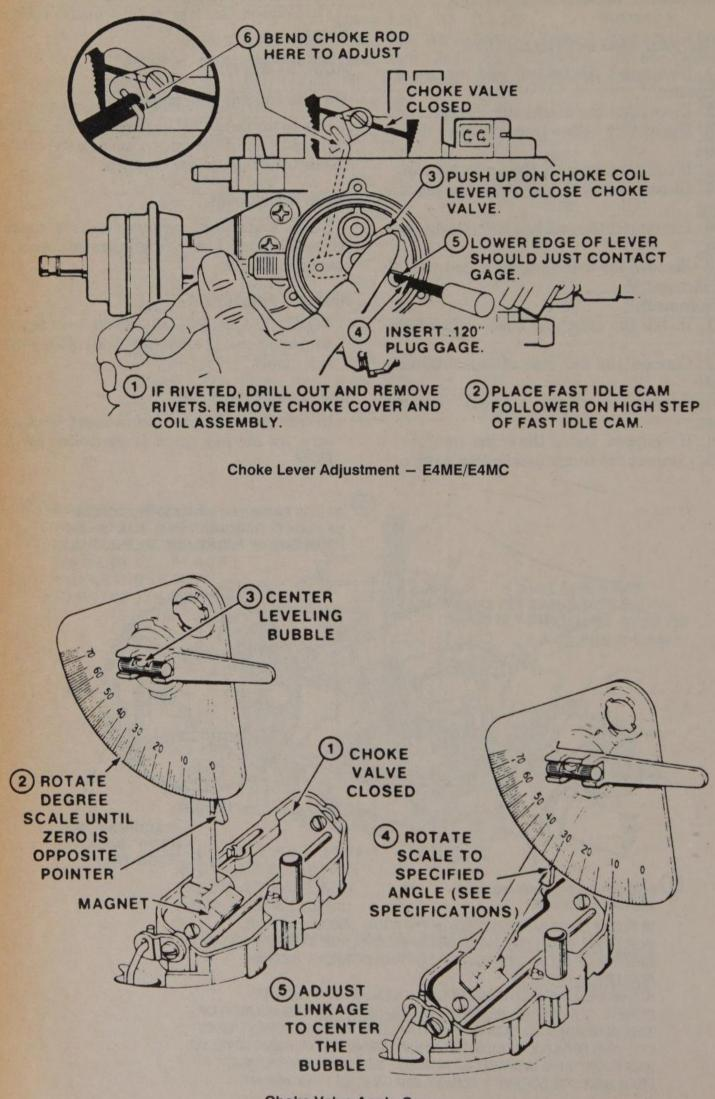
**Choke Valve Angle Gauge**
