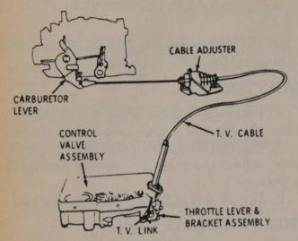
**Throttle Valve Cable Adjuster**
