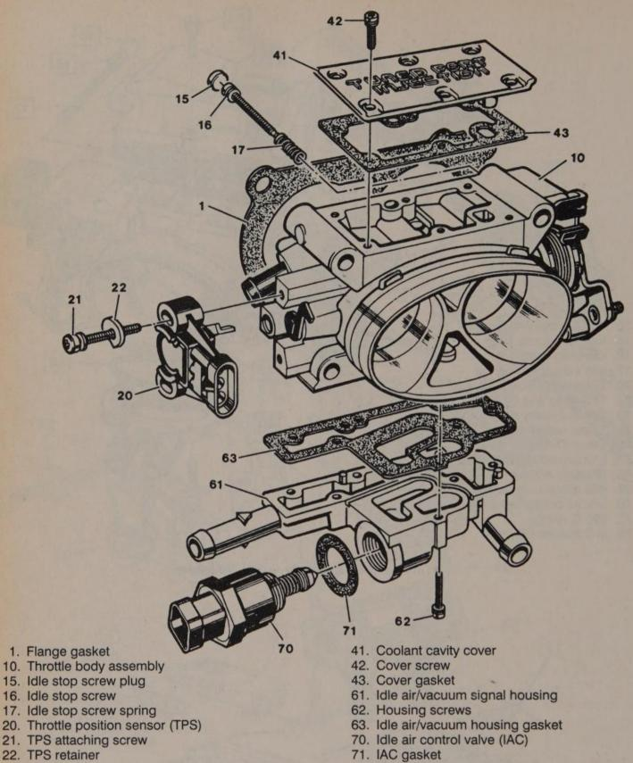
Throttle body assembly - 5.0L and 5.7L V8 engines
