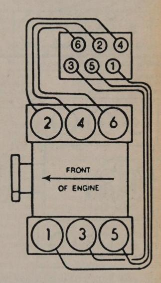
Buick-built V6 with C<sup>3</sup> ignition system; Engine firing order 1-6-5-4-3-2
