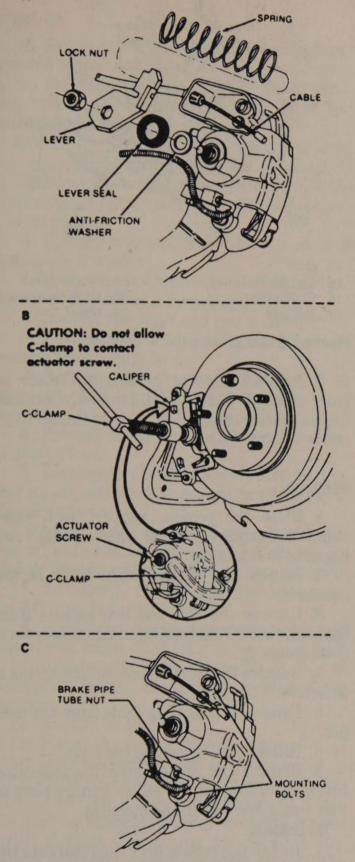
Remove and install rear caliper - 1982-88
