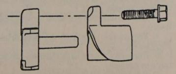
Door hinge spring compressor tool
