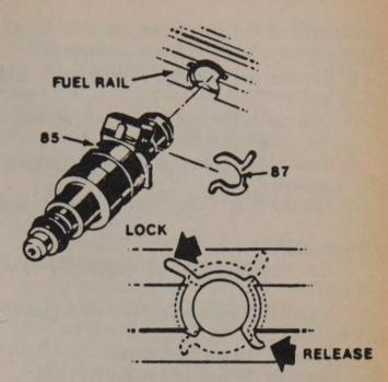
Removing fuel injector from the fuel rail
