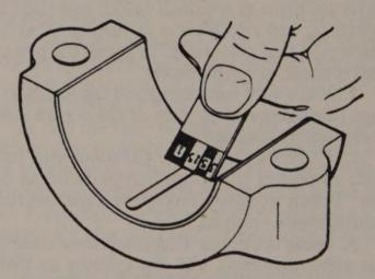
Measure the main bearing clearance by comparing the flattened strip to the Plastigage<sup>®</sup> scale as shown
