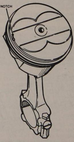
Install the pistons with the notch facing the front of the engine
