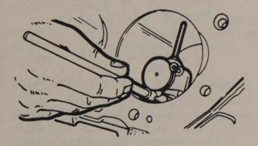
Measuring the cylinder bore with a dial gauge
