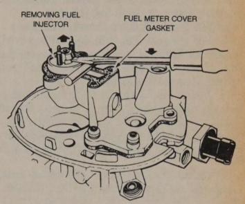
Removing the fuel injector
