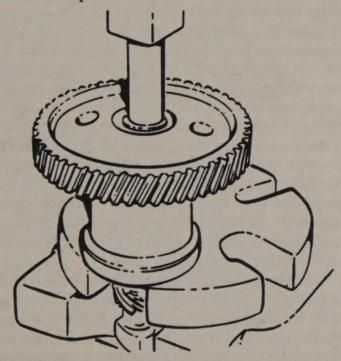
Pressing the timing gear from the camshaft – 4 cylinder
