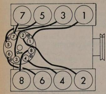
Chevrolet-built V8 engines; Engine firing order 8-4-3-6-5-7-2-1 Distributor rotation; clockwise
