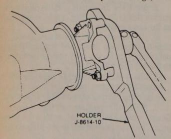
Rear axle pinion nut removal and installation
