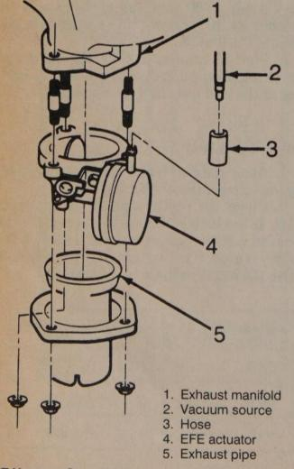
The vacuum servo type consists of a valve in the exhaust manifold and a Thermo Vacuum Switch (TVS) mounted on the engine coolant outlet housing.
