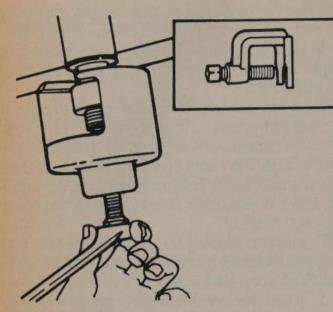
Using a tie rod puller
