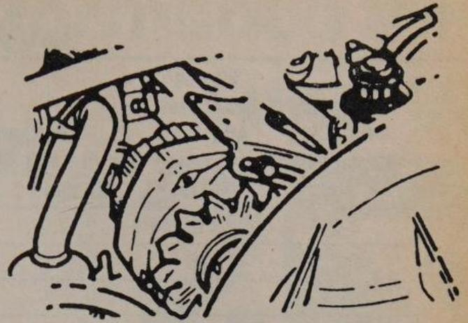
Alternator bracket location for final battery jumper cable connection
