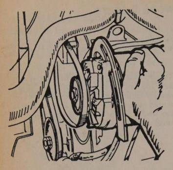
Push the component toward the engine and slip off the belt
