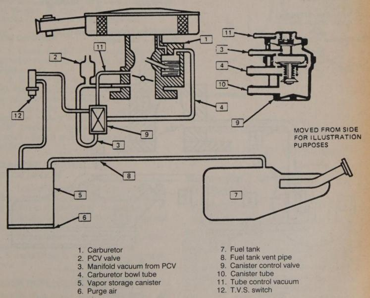
Evaporative Emission Control System (EECS) - 5.0L engine
