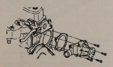
2. Install the heater hose and lower radiator hose to the water pump. Tighten the clamps to 15 ft. lbs. (20 Nm).
