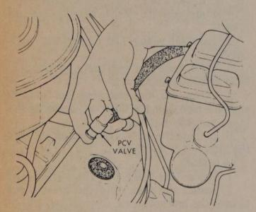
Pulling out the PCV valve from the rocker cover
