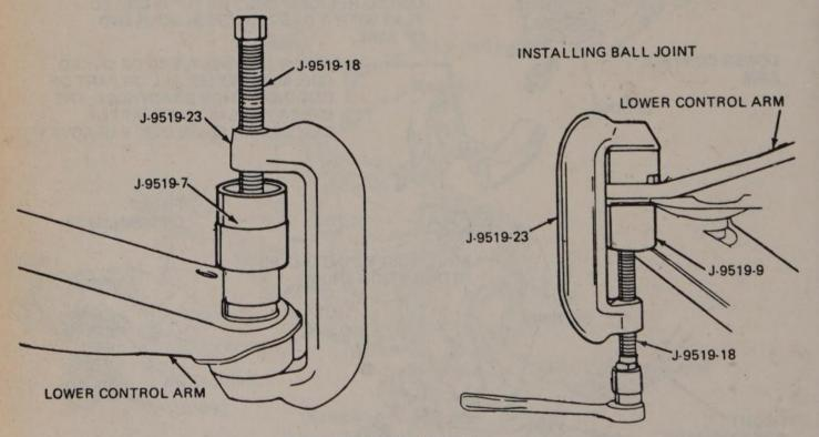
Remove or install ball joint
