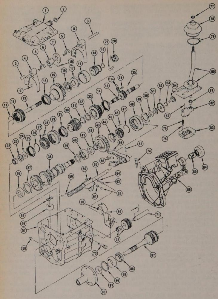
Exploded view of the 77mm 5-speed transmission
