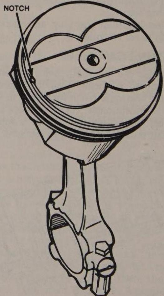
Install the pistons with the notch facing the front of the engine
