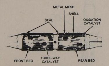
Cutaway view of the typical three-way catalytic converter There are essentially two types of catalytic converters: an oxidizing type and a three-way type. The oxidizing type requires the addition of oxygen to spur the catalyst into reducing the engine's HC and CO emissions into  $H_2O$ and  $CO_2$ . The oxidizing catalytic converter, while effectively reducing HC and CO emissions, does little, if anything, in the way or reducing NOx emissions. Thus, the three-way catalytic converter.
