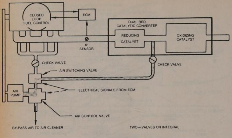
Air Injection Reaction System - Warm Engine
