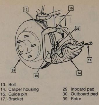
Removing rear brake pads - 1989-90
