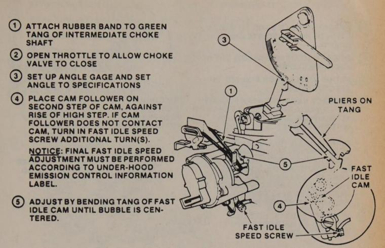
Choke Rod-Fast Idle Cam Adjustment - E4ME/E4MC
