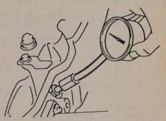
The screw-in type compression gauge is more accurate
