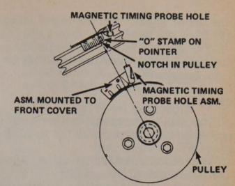
View of the timing marks, located at the front of the engine
