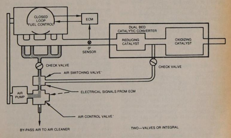
Air Injection Reaction System - Cold Engine
