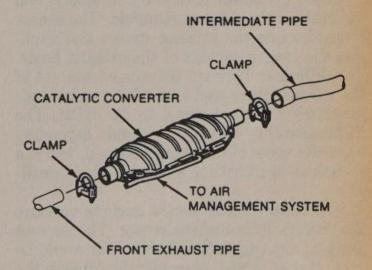
The catalytic converter is upstream of the muffler
