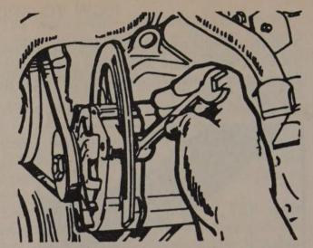
To adjust belt tension or to replace belts, first loosen the component's mounting and adjusting bolts slightly.
