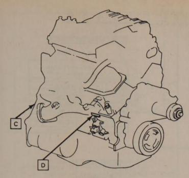
C. VIN code D. VIN derivative 3.1L V6 engine VIN code location
