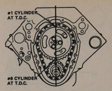
Timing sprocket alignment – V8. On V6, the #4 cylinder mark will align with the crankshaft sprocket
