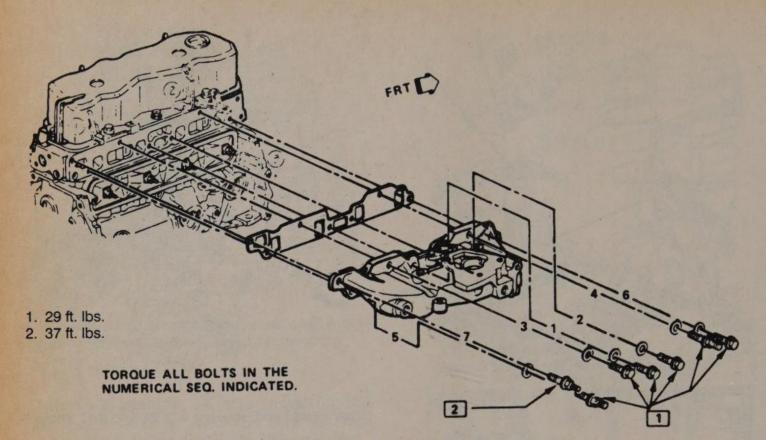
Intake manifold bolt tightening sequence for the 2.5L engine.
