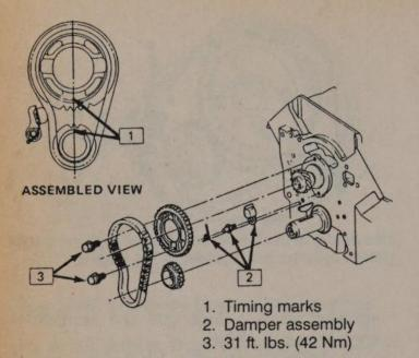
Timing chain and gear alignment – 3.8L Turbo engine
