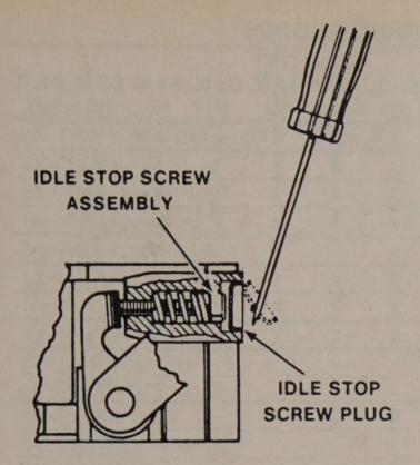
Removing the throttle stop screw plug-tuned port injection
