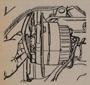
Slip the new belt over the pulley
