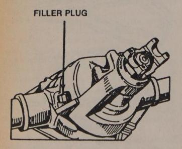
Remove the filler plug to check the lubricant level in the rear axle
