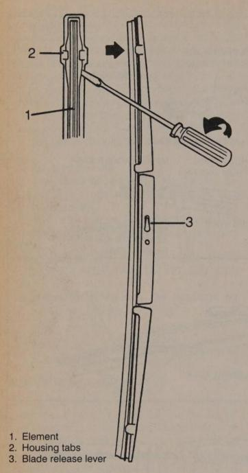
The rubber element can be changed without replacing the entire blade assembly
