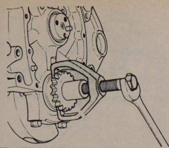
V6 and V8 crankshaft sprocket removal
