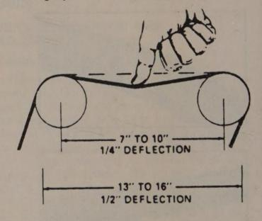
A gauge is recommended, but you can check belt tension with thumb pressure
