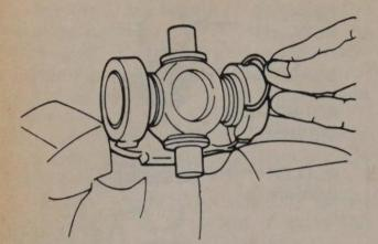
Installing trunnion snap ring
