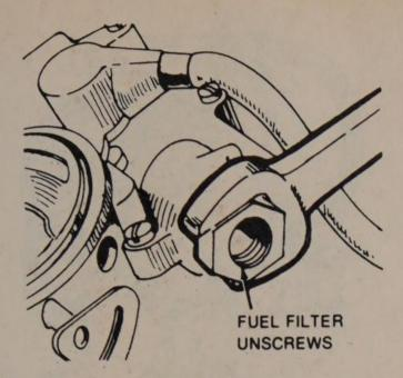
Removing the fuel filter retainer
