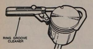
Cleaning the piston ring grooves using a ring groove cleaner
