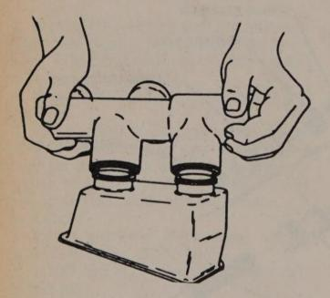
Install the master cylinder to the reservoir with a rocking motion
