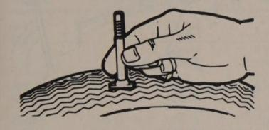
Tread depth can be checked with an inexpensive gauge
