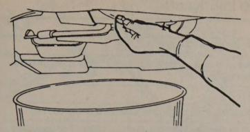
By keeping inward pressure on the plug as you unscrew it, oil will not escape past the threads
