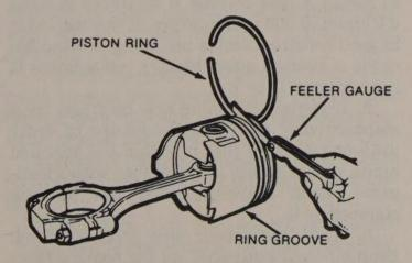
Check the piston ring side clearance
