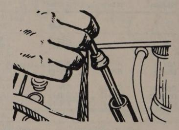
The oil level is checked with the dipstick
