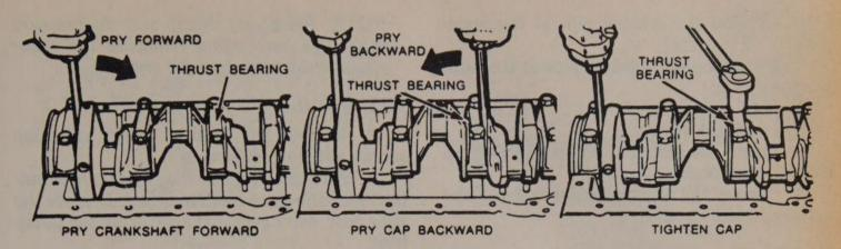
Align the thrust bearing as illustrated. Torque the caps to specifications.
