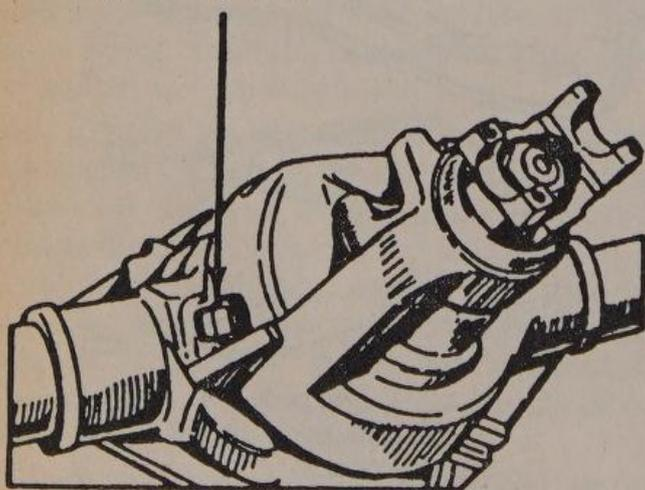
Remove the filler plug to check the lubricant level in the rear axle
