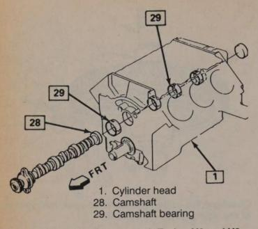
Camshaft and bearings – 3.8L Turbo, V6 and V8 engines similar
