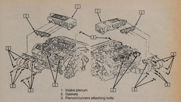
Intake plenum and runners - Tuned Port Injected engines
