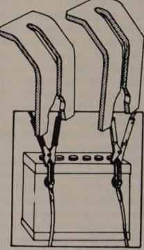
Side terminal batteries oc casionally pose a problem when connecting jumper cables. There frequently isn't enough room to clamp the cables without touching sheet metal .Side terminal adaptors are available to alleviate this problem and should be removed after use.
