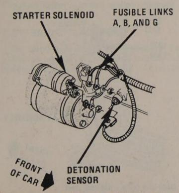
Fusible link A, B and G – located at the starter motor
