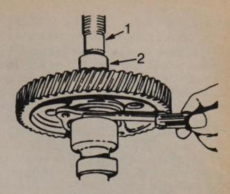
Checking the camshaft clearance upon installation of the timing gear – 4 cylinder
