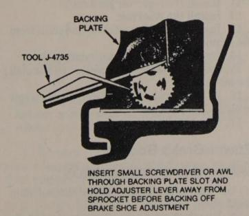
Adjusting rear drum brakes using brake adjusting spoon
