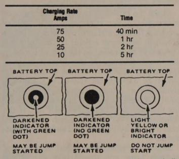
Maintenance-free batteries contain their own built in hydrometer
