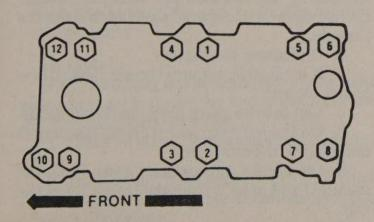
Lower intake manifold torque sequence – V8 engines with TPI
