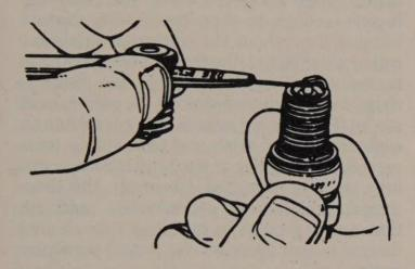
Always use a wire gauge to check the electrode gap
