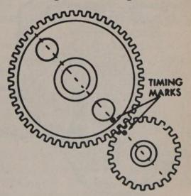
Timing gear alignment inline 4 cylinder
