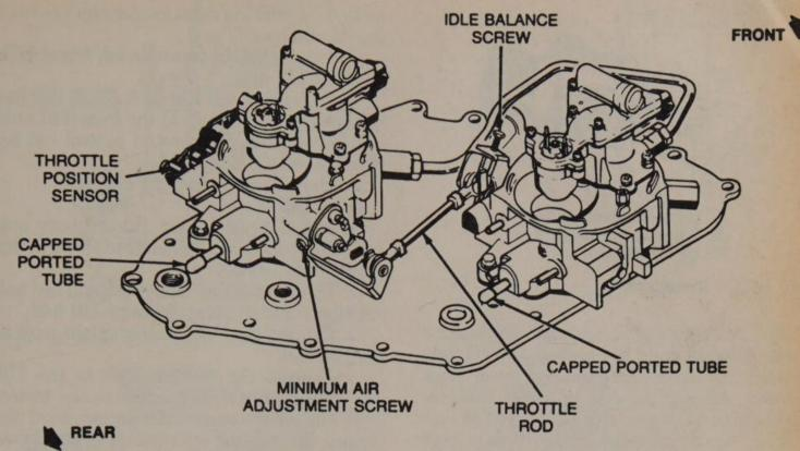
Cross-Fire Injection System (CFI) - Twin throttle Body Injectors (TBI)
