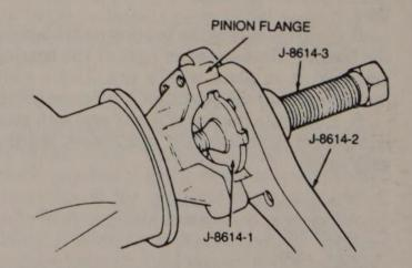
Rear axle pinion oil seal installation
