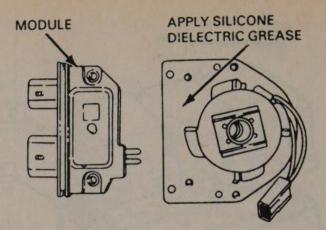
Remote coil ignition module – always coat the base with silicone dielectric grease
