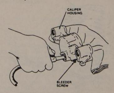
Use air pressure to remove the piston from the bore
