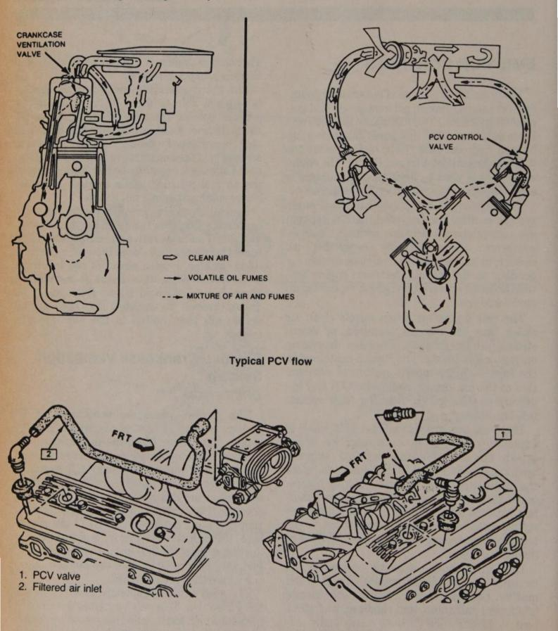
4. Shut off the engine. Shake the valve and listen for the rattle. If valve does not rattle, replace it.
