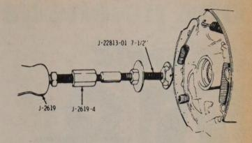
**Removing the Rear Axle Bearing**
