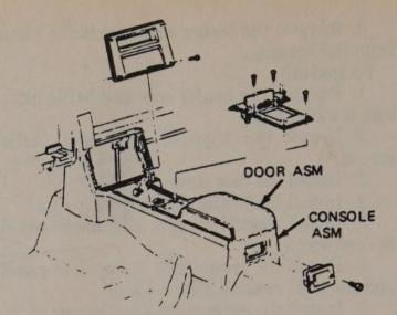
Console, radio and A/C/heater control trim servicing
