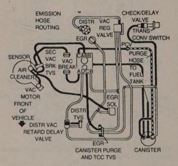
1982 6-2.8L engine with automatic transmission
