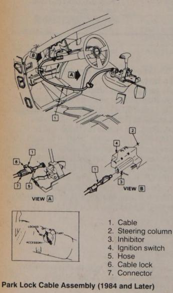
steering column slider and disconnect the cable.
