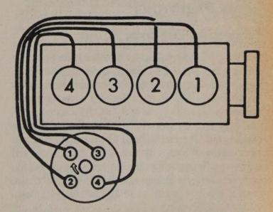
Pontiac-built 4–151 (2.5L) engine; Engine firing order; 1-3-4-2 Distributor rotation; clockwise
