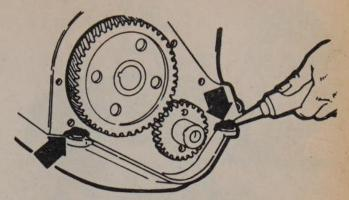
Use sealer at the timing cover-to-oil pan and the oil pan-to-cylinder block joints; 4-151 engine
