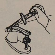
Check the valve spring test pressure
