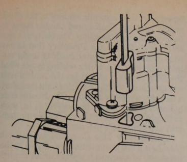
Plug the idle passages of each throttle body as shown
