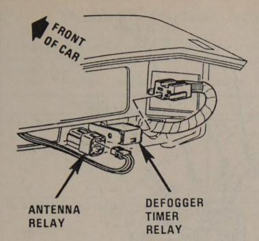
Antenna and rear defogger relay – RH side of instrument panel
