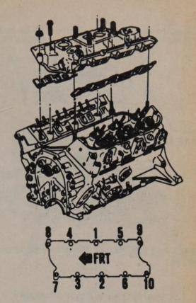
Intake manifold bolt tightening sequence for the 173-V6 engine
