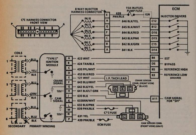
C<sup>3</sup>I system wiring
