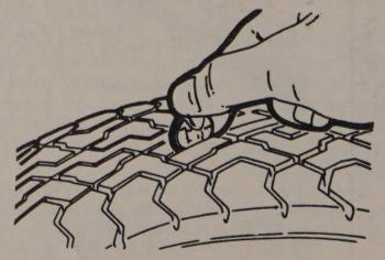
A penny works as well as anything for checking the tire tread depth; when you can see the top of Lincoln's head, its time for a new tire.
