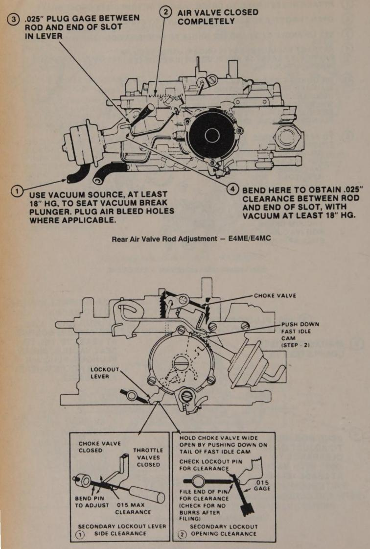
Secondary Lockout Adjustment - E4ME/E4MC
