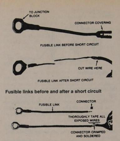
New fusible links are spliced to the wire
