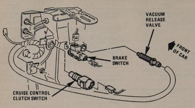
Brake light switch-mounted above brake pedal
