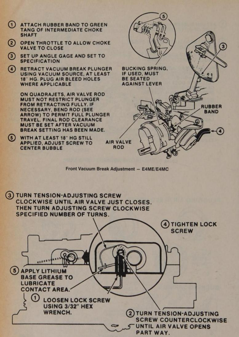
Air Valve Spring Adjustment - E4ME/E4MC
