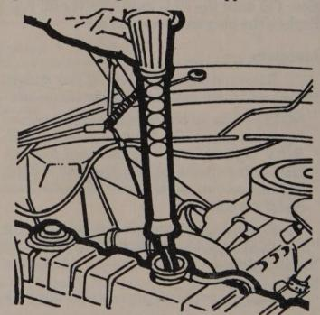
Coolant protection can be checked with a simple float-type tester
