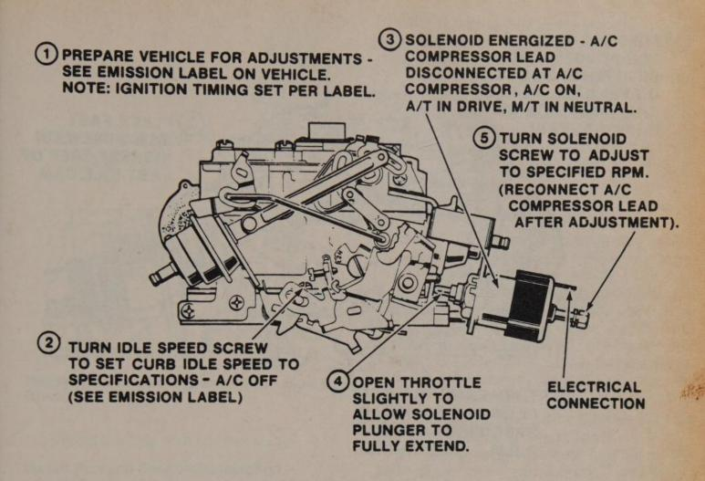
idle speed adjustment-with A/C
