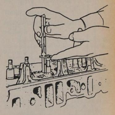
Checking valve spring installed height
