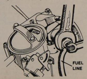
The fuel filter is located behind the large fuel line inlet nut on the carburetor
