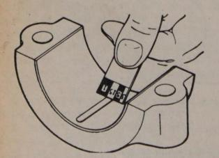
Measure Plastigage® to determine bearing (rod or main) clearance
