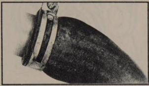
A good test for any hose is to feel it for soft or spongy spots. Frequently these will appear as swollen areas of the hose. The most likely cause is oil soaking. This hose could burst at any time, when hot or under pressure.
