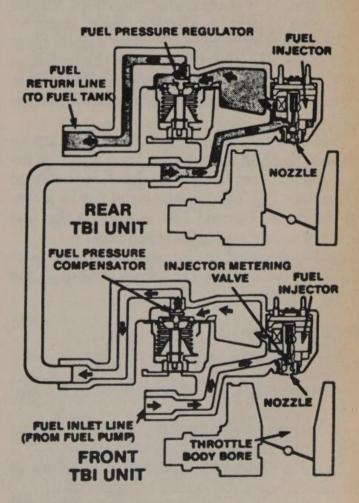
TBI's fuel flow schematic CFI System
