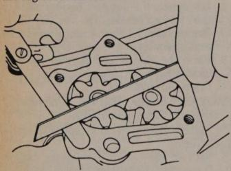
Measure the oil pump and clearance with a feeler gauge and straightedge
