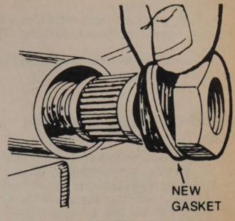
Install the new filter and spring. Certain early models use a bronze filter element but most are made of paper
