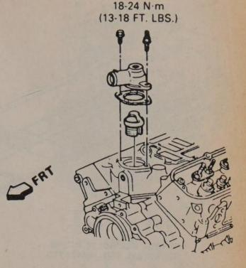
Thermostat and housing - 2.8L and 3.1L engine
