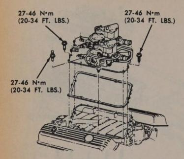
TBI plate and gasket installation on V8 engines so equipped
