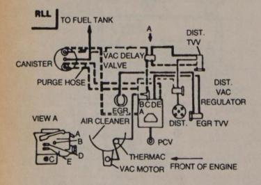
1982 4–2.5L engine with manual trans. and no A/C
