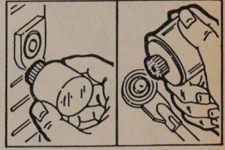
A special tool is available for cleaning the side terminals and clamps
