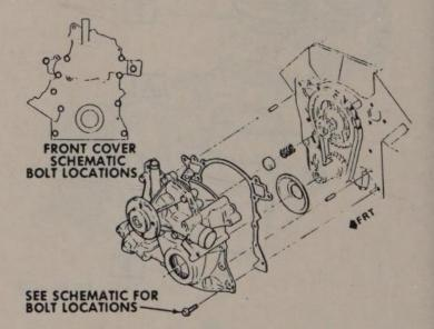
Front timing cover - 3.8L Turbo engine
