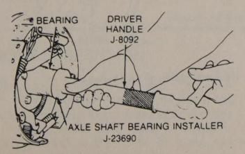
Installing the Rear Axle Bearing
