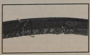
This belt has deep cracks, which cause it to flex. Too much flexing leads to heat build-up and premature failure. These cracks can be caused by using the belt on a pulley that is too small. Notched belts are available for small diameter pulleys.
