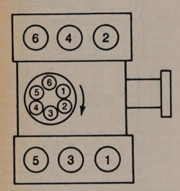
Chevrolet-built 6–173 (2.8L) engine; Engine firing order; 1-2-3-4-5-6 Distributor rotation; clockwise
