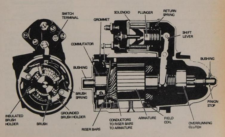
Cross section of a typical starter
