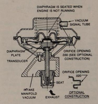
Cross section of a negative backpressure EGR valve
