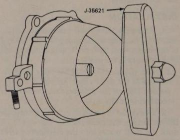
One piece rear seal installation with tool
