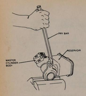
Removing the mast cylinder reservoir
