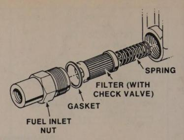
Fuel filter - carbureted engines
