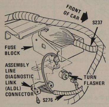
Turn signal flasher – located near the fuse block – late model
