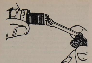
Adjust the electrode gap by bending the side electrode
