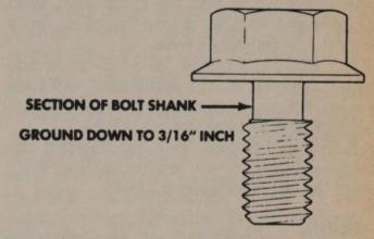
Special bolt is used to aid in the oil pan removal
