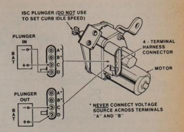
Idle speed control E4ME and E4MC carburetors
