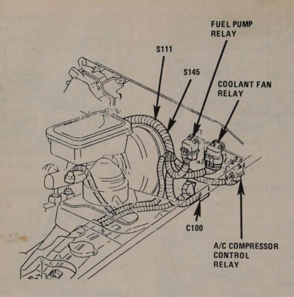
Fuel pump, coolant fan, A/C compressor relay - LH side of power brake booster
