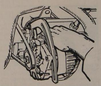
Pull outward on the component and tighten the mounting bolts
