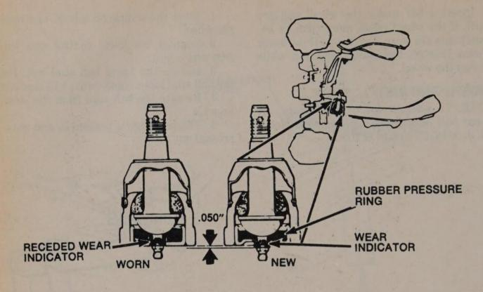
Wear indicator used on the lower ball joints - all models
