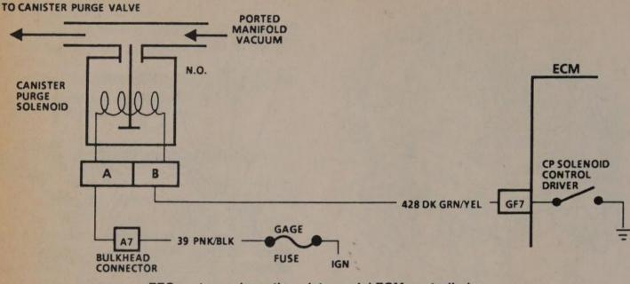
EEC system schematic - late model ECM controlled
