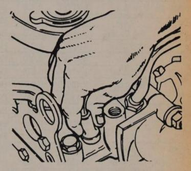
Twist and pull on the rubber boot to remove the spark plug wires; never pull on the wire itself
