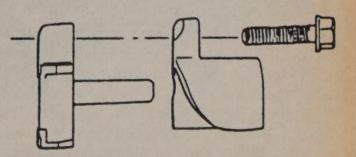
Transmission identification – early model 4 and 5-speed 77mm manual transmission
