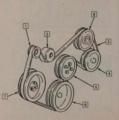
Belt routing - 1990 3.1L engine with manual transmission
