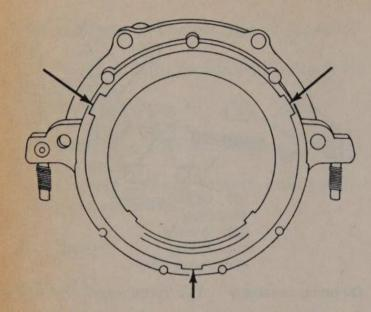
One piece rear main seal – use prybar in slots to remove
