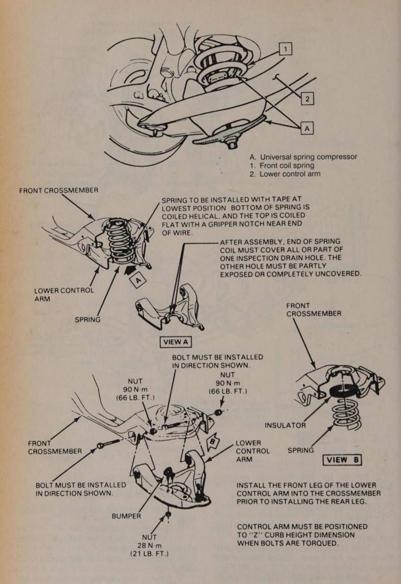
6. Install a universal spring compressor and compress the spring.
