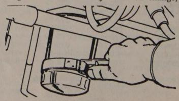
Remove the oil filter with a strap wrench
