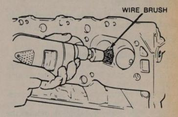
Remove the carbon from the cylinder head with a wire brush and electric drill
