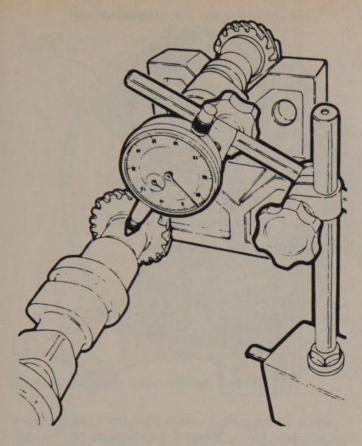
Check the camshaft for straightness
