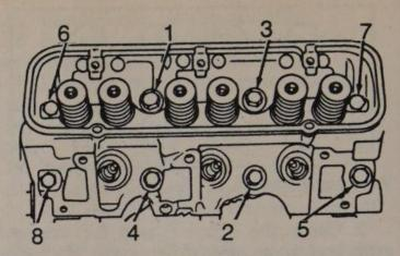
Torquing sequence for the 3.8L Turbo engine
