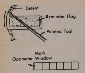
Resetting the emission odometer flag
