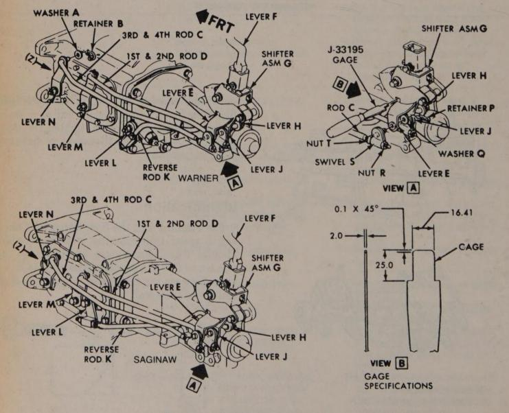
Transmission shift linkage adjustment
