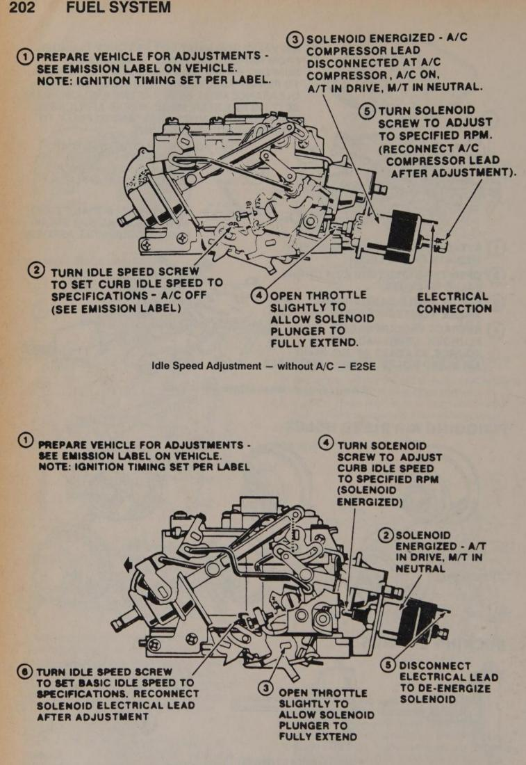
Idle Speed Adjustment - with A/C - E2SE
