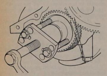
The inline 4-cylinder crankshaft gear is removed with a gear plier
