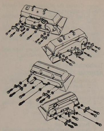
Exhaust manifold installation
