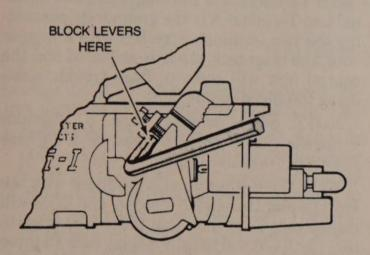
Block throttle lever movement as shown
