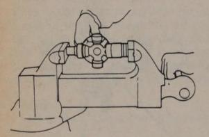
Installing U-joint trunnion seal
