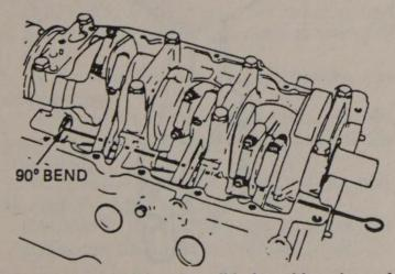
Aligning camshaft bearing oil holes with a piece of wire bent at a 90° angle. The holes MUST be in alignment
