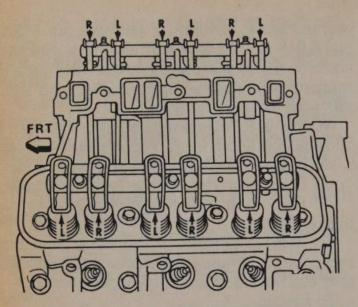
Rocker arm positioning -- 3.8L Turbo, each rocker arm is marked with a R or L, used for location
