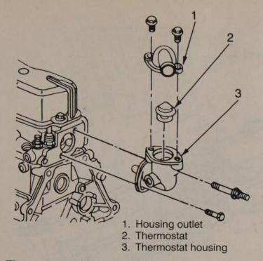
Thermostat and housing – 2.5L engine
