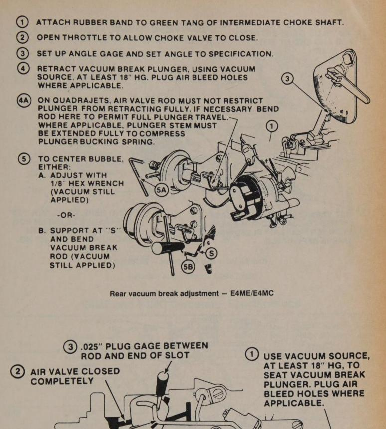
BEND ROD HERE TO ADJUST GAGE CLEARANCE TO .025", WITH VACUUM AT LEAST 18" HG.
