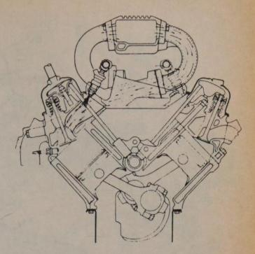
**Cross section view of Tuned Port Injection Systems**
