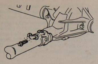
Strap-type retainer on drive shaft
