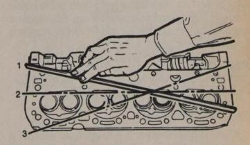
Check the cylinder head for warpage
