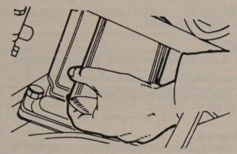
Install the new oil filter by hand
