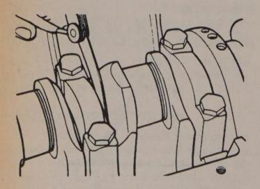
pry the crankshaft the extent of its axial travel several times, holding the last movement toward the front of the engine. Add thrust washers if required for proper alignment. Torque the thrust bearing cap to specifications.
