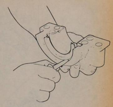
Rear main seal - removing lower half
