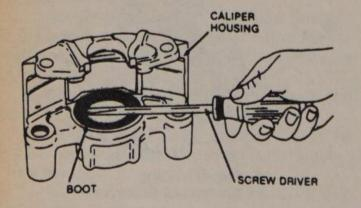
Remove the piston boot with an awl
