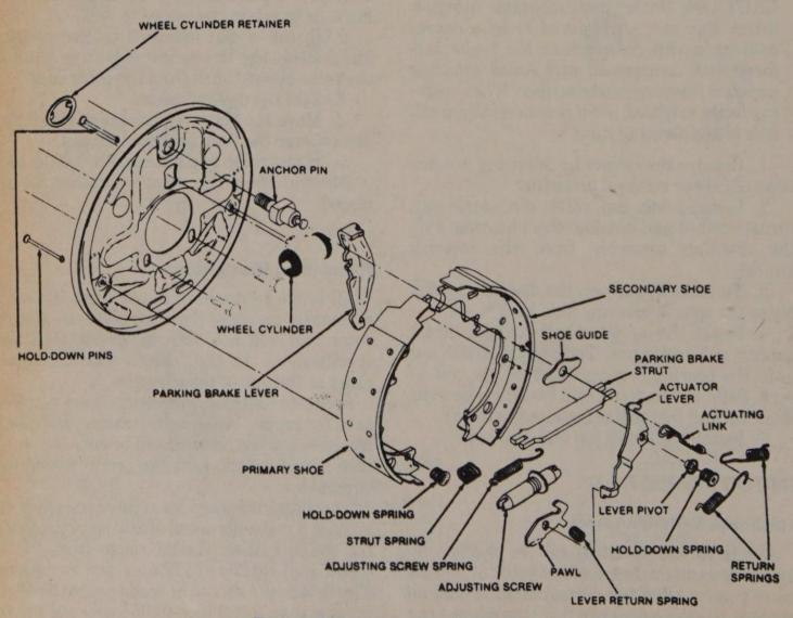
Exploded View of the Rear Brake Drum
