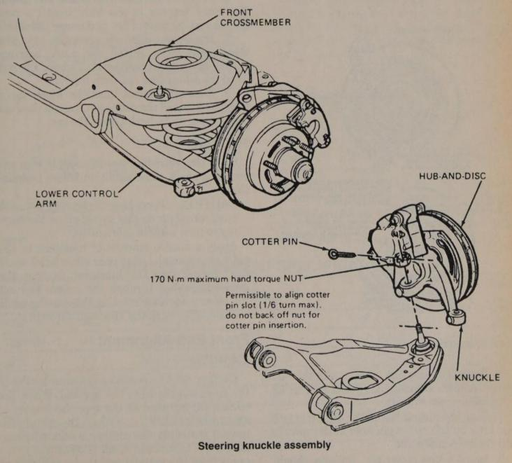
6. Remove the 2 bolts securing the strut to the steering knuckle and remove the steering knuckle.
