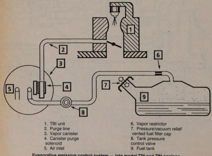
Evaporative emission control system - late model TPI and TBI engines
