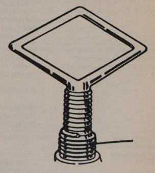
Screw the threaded insert onto the installation tool until the tang engages the slot. Screw the insert into the tapped hole until it is 1/4-1/2 turn below the top surface. After installation break off the tang with a hammer and punch
