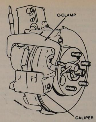
Install a C-clamp to retract the brake pads
