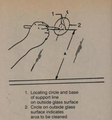
Locating and marking bonded rear view mirror support on the glass
