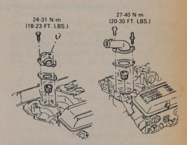
Thermostat and housing - V8 engines
