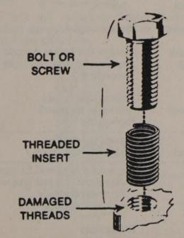
Damaged bolt holes can be repaired with thread repair inserts
