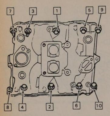
Intake manifold torque sequence – 1989 3.8L Turbo engine
