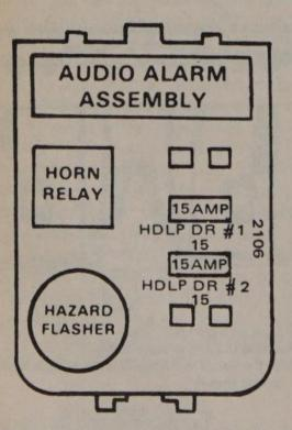
Convenience center – located under the instrument panel on the right side of steering column. The two headlight door fuses are located in the convenience center
