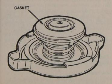
Check the condition of the radiator cap gasket
