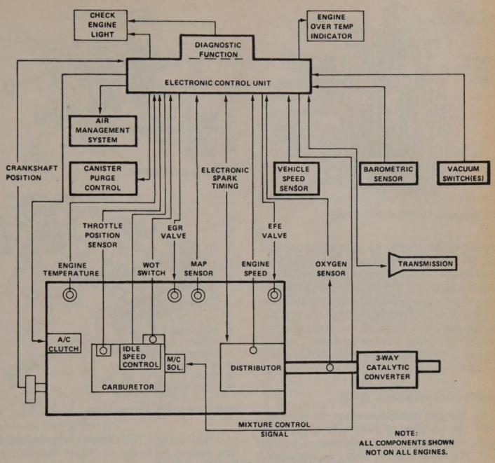
**Computer Control Command schematic**
