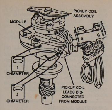
Ohmmeter 1 shows the connections for testing the pick-up coil. Ohmmeter 2 shows the connections for testing the pick-up coil continuity
