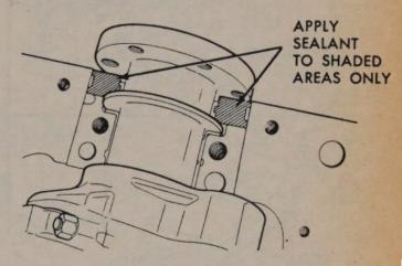
Sealing upper and lower main seal halves
