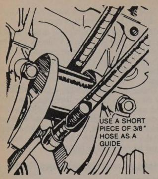
Use lengths of vacuum hose or rubber tubing to protect the crankshaft journals and cylinder walls during piston installation
