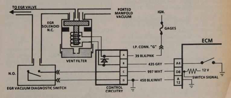
ECM and vacuum operated EGR valve schematic
