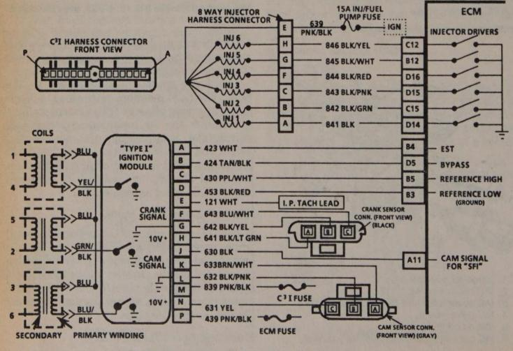
Electronic spark timing 6-3.8L Turbo with C<sup>3</sup>I ignition
