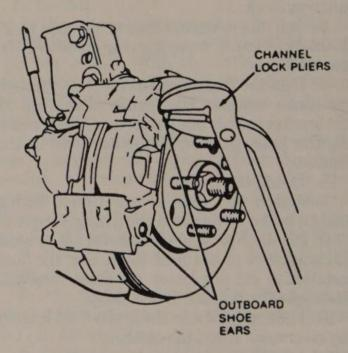
Bend the outboard pad ears into place with a large pair of slipjoint pliers
