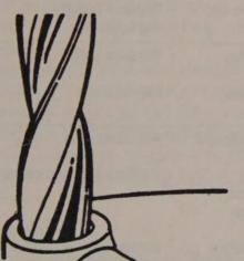
Before effecting a repair to a threaded hole, remove any snapped, broken or damaged bolts or studs. Penetrating oil can be used to free frozen threads. The offending item can be removed with locking pliers or with a screw or stud extractor. After the hole is clear, the thread can be repaired, as shown in the series of accompanying illustrations.
