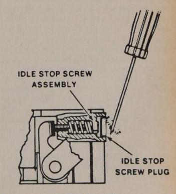
Removing the Idle Stop Screw Plug
