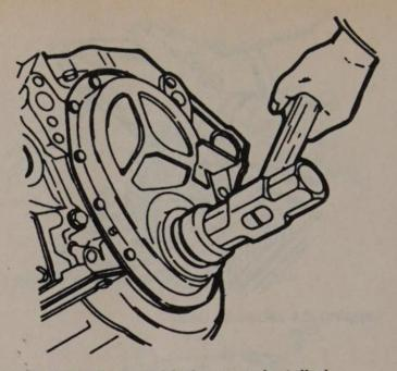
Oil seal installation with the cover installed
