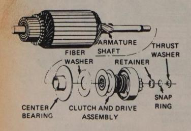
Starter and drive assembly removed
