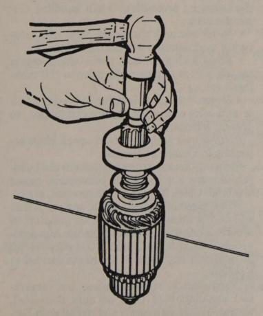
Use a piece of pipe to drive the retainer toward the snapring
