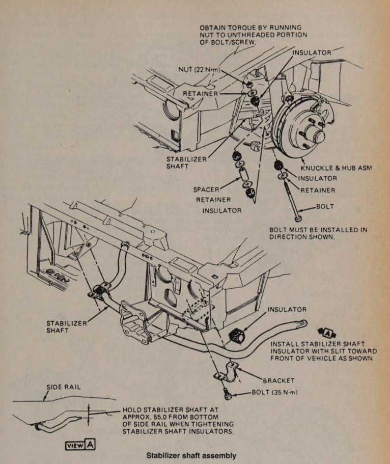
2. Remove the link bolt, nut, grommet, spacer and retainers.
