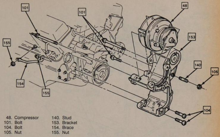
A/C compressor - V8 engines with serpentine belt
