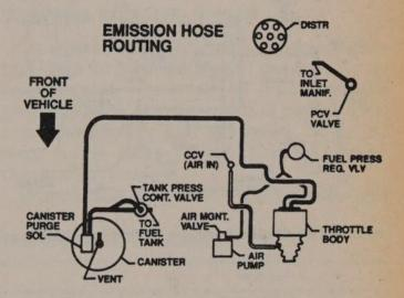
1990 6–3.1L engine (VIN T) with manual trans – automatic trans. does not have an AIR pump
