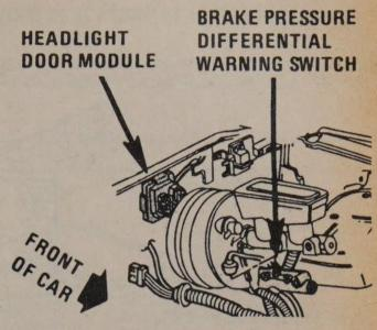
Headlight door module – behind brake power booster
