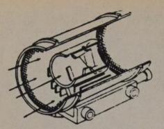
Section view of Air Mass Flow Sensor
