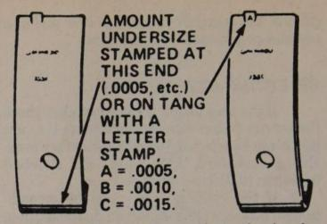
Undersize marks are stamped on the bearing shells. The tang fits in the notch on the rod and cap
