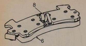
6. Inboard shoe & lining8. Shoe retainer spring
