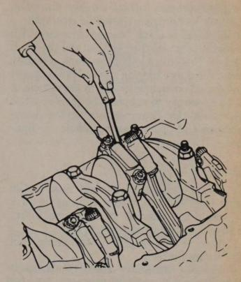
Check the connecting rod side clearance with a feeler gauge. Use a small pry bar to carefully spread the rods to specified clearance
