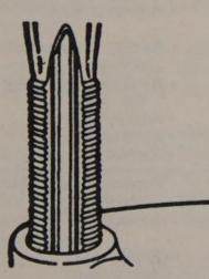
With the tap supplied, tap the hole to receive the thread insert. Keep the tap well oiled and back it out frequently to avoid clogging the threads
