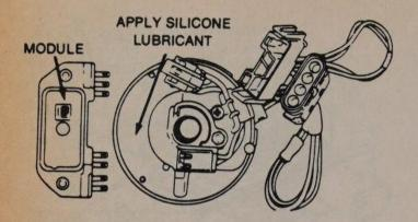
Module replacement; be sure to coat the mating surfaces with silicone lubricant
