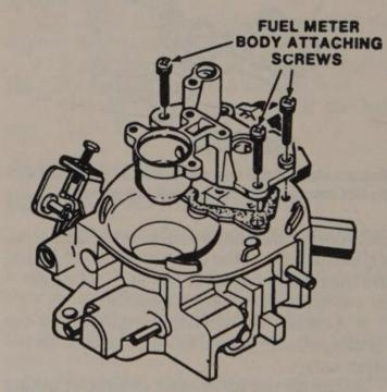
Fuel meter body attaching screws
