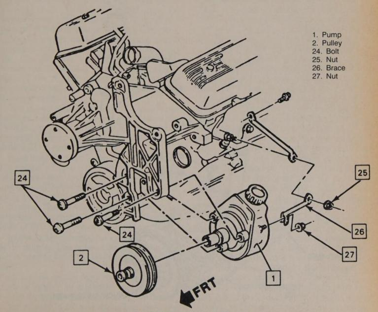
Power steering pump - V8 engine
