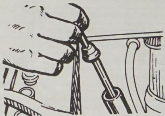
The oil level is checked with the dipstick
