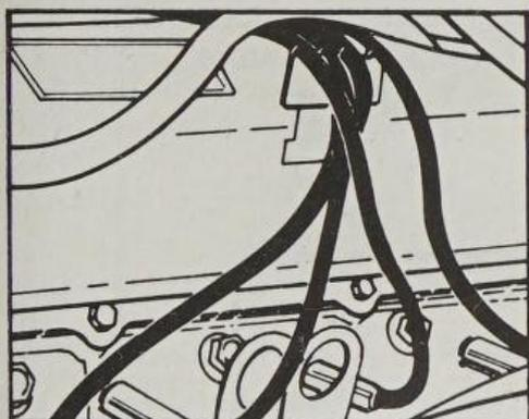
Misfiring can be the result of spark plug leads to adjacent, consecutively firing cylinders running parallel and too close together
