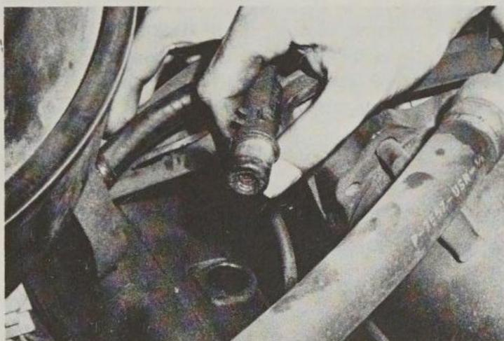
Pulling out the PCV valve from the rocker cover
